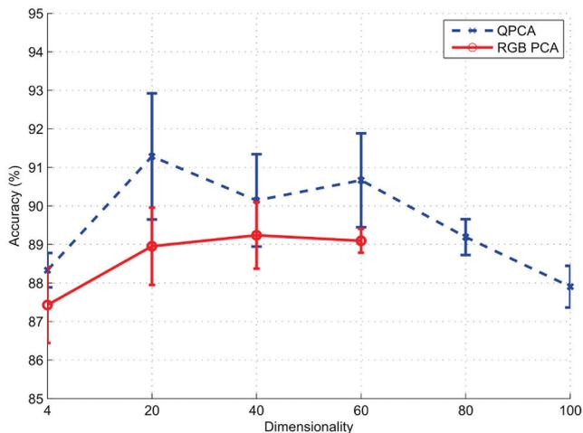
Fig. 2. Classification performance versus the local descriptor dimensionality for the UC Merced datasets. The bars on the plot represent one standard deviation. Since the maximal dimensionality of the RGB PCA-based descriptor is 75 we tested it up to 60-D
